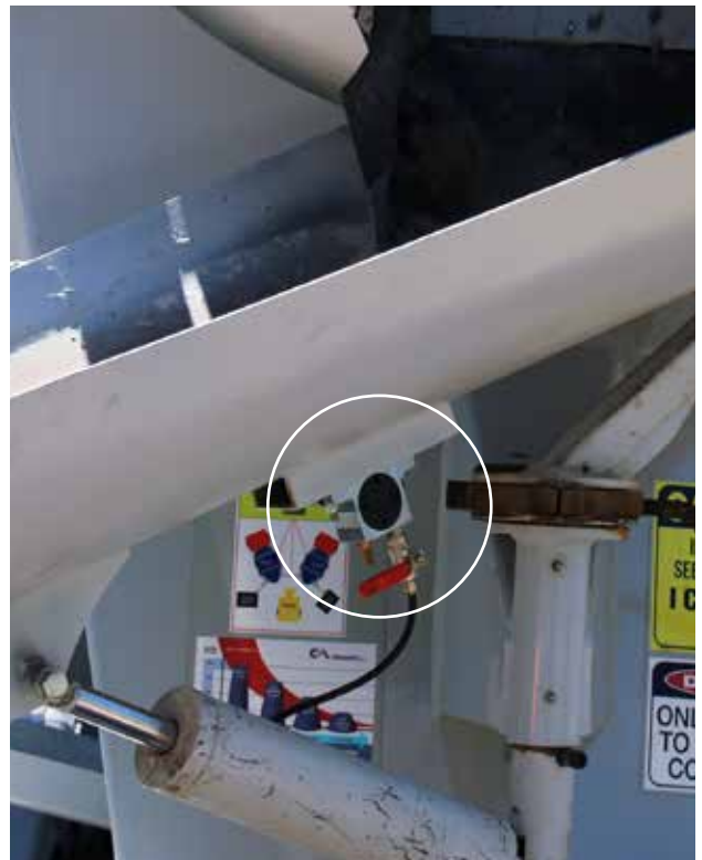
OT (rotary pneumatic vibrator) - Chute on concrete mixer
