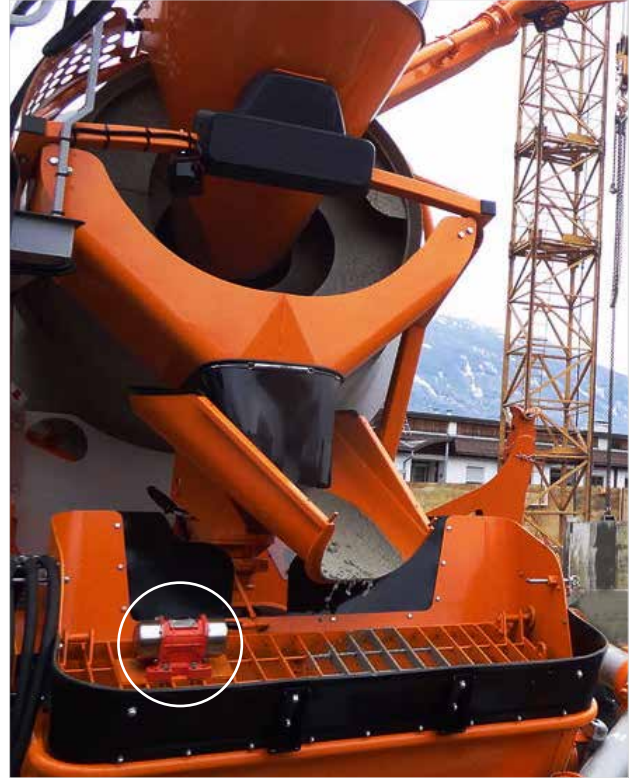
MVE-DC (electric vibrator) - Concrete pump
